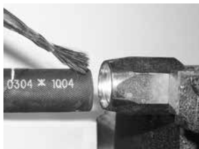
Apply lubricant to hose cover.
