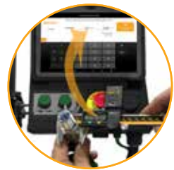
CrimpIQ™ controller supports bluetooth calipers to input crimp diameter measurements.
