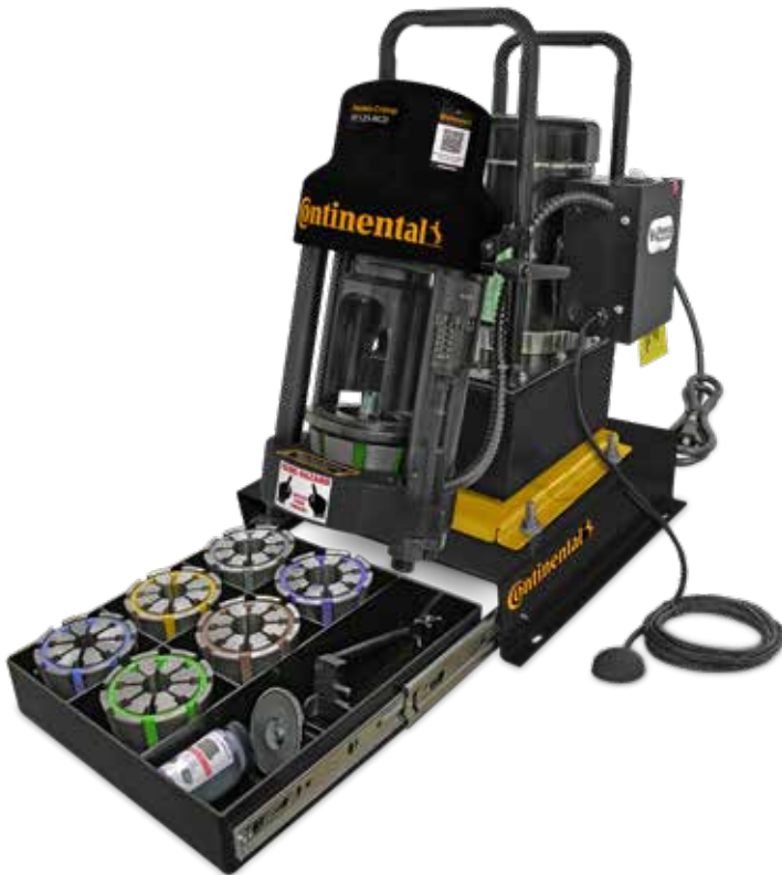
Coupling stop makes repetitive crimps faster.
