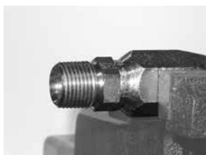
Stem properly seated against socket.
