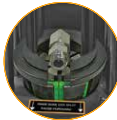
Ideal notched pressure plate when crimping 90° fittings.
