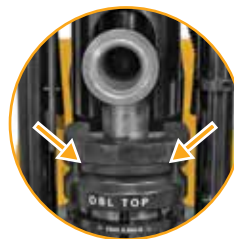
PC150 spacer kit ideal for crimping extra long elbow fittings.
