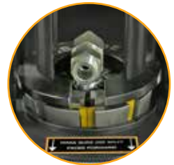
Ideal notched pressure plate when crimping 90° fittings.
