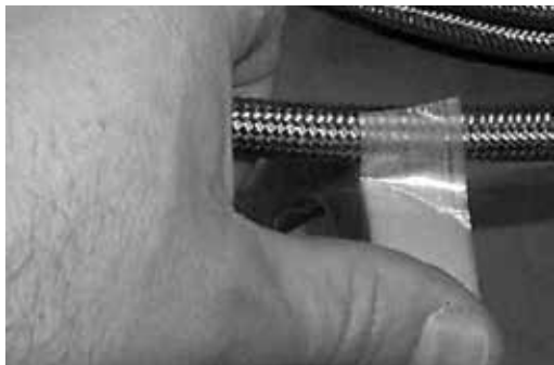
Tape hose before cutting.
