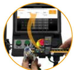
CrimplQ™ controller supports bluetooth calipers to input crimp diameter measurements.
