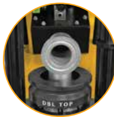
Open design allows the operator to accurately position the fitting prior to crimping.
