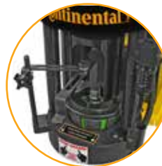
Coupling stop makes repetitive crimps faster.
